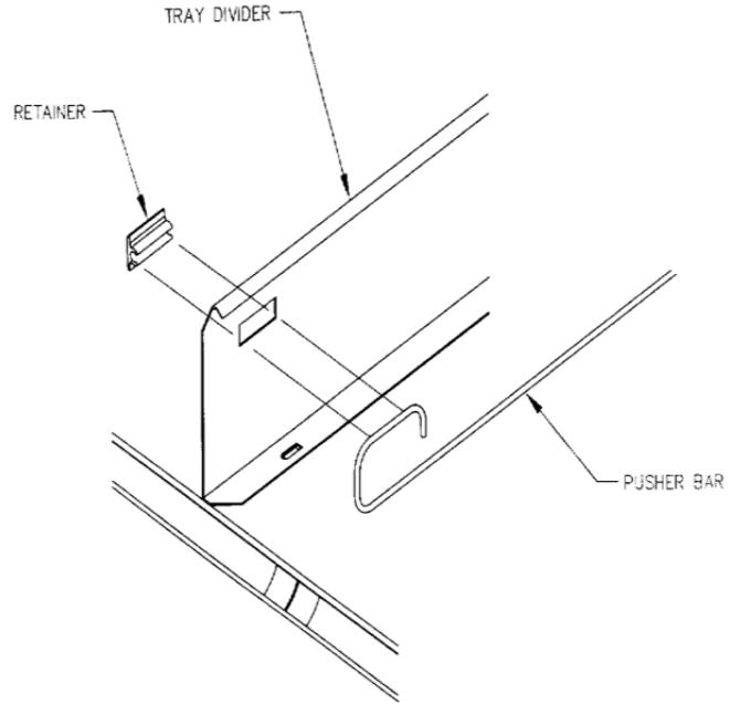
**Figure 5.2 Pusher Bar Installation**
