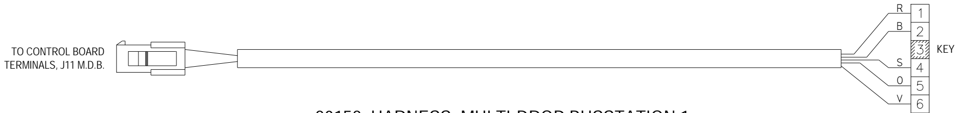
20158, HARNESS, MULTI-DROP BUSSTATION 1
